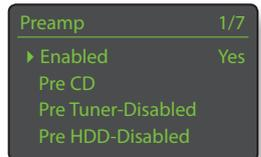
Inputs can be enabled, disabled and renamed and, as "virtual" NDX/5XS inputs, can be assigned to NDX/5XS handset input keys.
