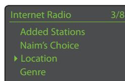
Once a station is selected the NDX/5XS display will exit from **list mode** and revert to normal mode. To re-enter list mode for further list browsing and selecting press the handset **ok/list** key.
