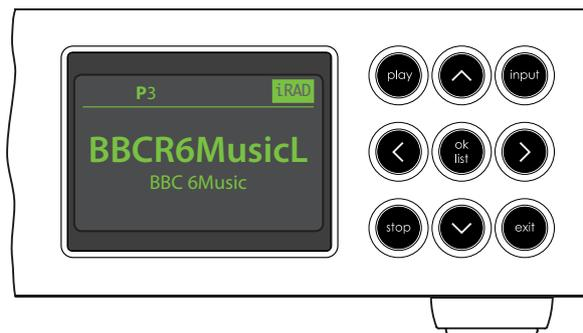
In normal play mode the NDX/5XS screen provides a variety of information on the current setup, the input selected and the material playing. A typical normal play mode screen is illustrated above showing the internet radio station BBC 6Music playing.
