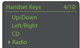
Beneath the **Up/Down** keys and **Left/Right** keys parameters the **Handset Keys** menu displays a list of the eight handset input keys. Selecting one of the keys then displays a list of the four existing assignments to that key (including unassigned). To change an assignment, select the assignment number to be altered and, from the subsequent menu, select the desired input.
