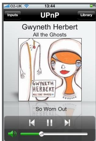
The **Playing** screen displays the currently playing item and provides appropriate transport controls. When a Radio station is playing an icon is also provided to open a preset station menu through which presets can be either stored or recalled.
