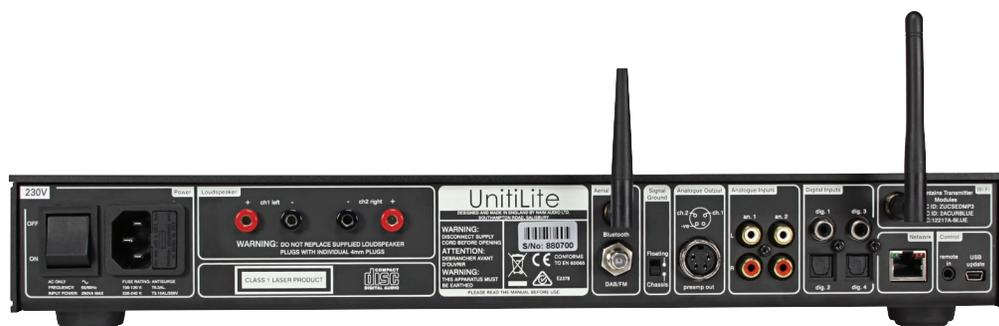
**Two aerials, no less, for Wi-fi and Bluetooth, attest to the UnitiLite's comms. skills. There is a network RJ45 socket, S/PDIF inputs, loudspeaker outputs and more, underscoring just how capable this Naim is.**
