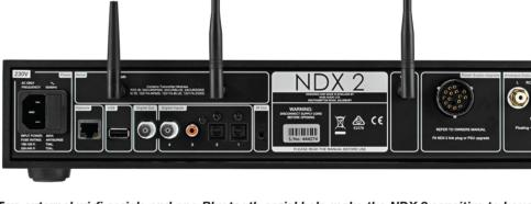
Two external wi-fi aerials and one Bluetooth aerial help make the NDX 2 sensitive to household router and phone signals, aiding data speeds and reception stability. There is an array of digital inputs and Naim's DIN socket output at right, but no XLR balanced outputs from the DAC.
