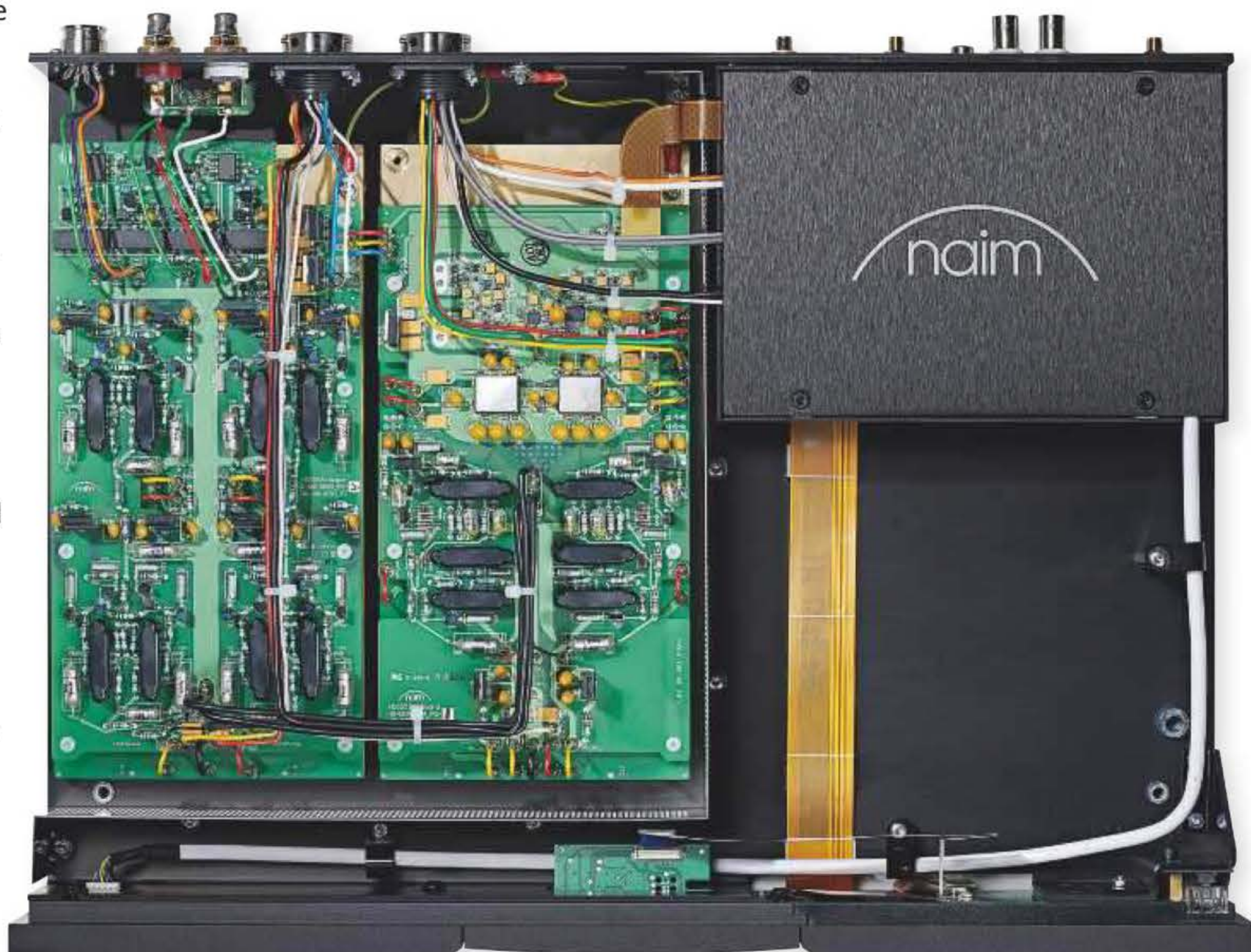
RIGHT: Naim's DAC board [centre] and analogue filter/output board [left] are both mounted on sprung-suspended brass plates while the two PCM1704 DAC chips are separately screened [silver cans, centre]
