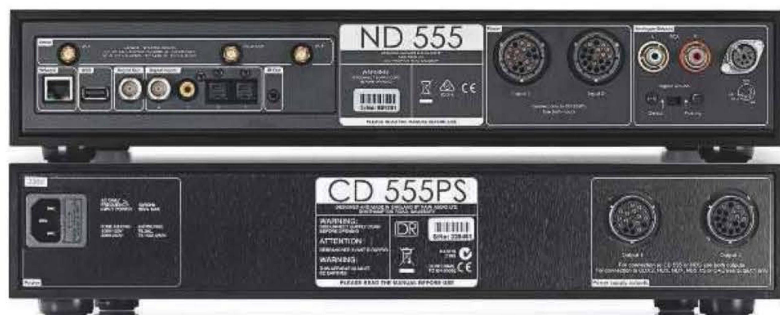
ABOVE: Two Toslink optical and coaxial digital ins (one on BNC) are joined by USB-A and wired/wireless Ethernet for network audio. Outputs are on RCAs and a 5-pin DIN. Note the two large connectors to accommodate the DR-series PSU [bottom]
